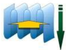
Vertical position favors the output of air and the pathway of water vapor
